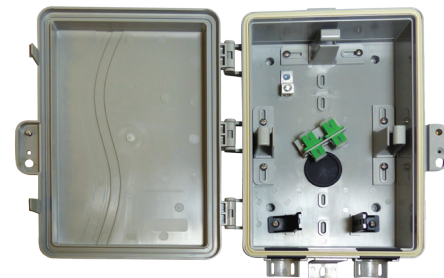
125-1299: w/2 SC/APC simplex adapters, hex bolt, 1 rear entry/2 flat grommets, gasket, PVC
